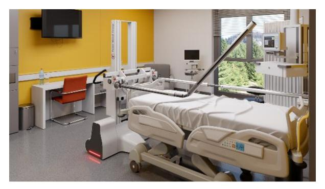
It only takes a few steps to get the system ready to go: Positioning at the foot of the bed, extending the supporting device, extending the winding shafts, securing the bedsheet with loop-and-hook fastening. (Image source: Franz Morat Group)
