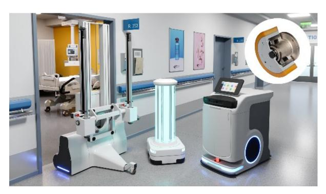
Wheel hub drives from the Framo Morat modular gearbox are used in various autonomous units such as disinfection robots and medical transportation vehicles – both in hospitals and in care facilities. (Image source: Franz Morat Group)
