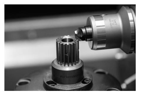
The Radial Gear Chamfering process takes place in an environmentally friendly way in dry cutting. Defined and reproducible chamfers on the front edges are also possible for complex components. (Image source: TEC for GEARS)
