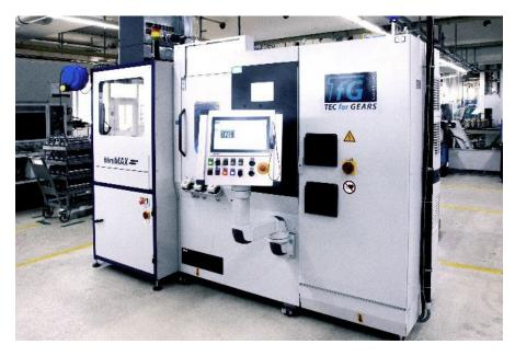
With a footprint of approx. 2 m<sup>2</sup>, the RGC 350 is extremely compact. Interlinking with a robot cell enables the machine to work virtually autonomously due to the reproducible results. (Image source: Framo Morat)
